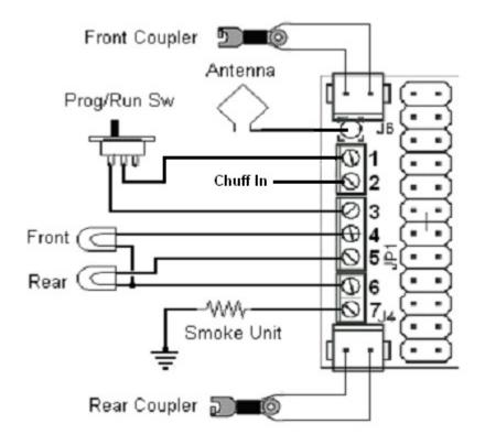
Trim the wires that go into the mini screw terminal strip to prevent stray strands of wire. Be sure that the screws in the mini terminals are turned counter-clockwise to open, before wiring. Do not over tighten terminal screws when attaching the wires.
