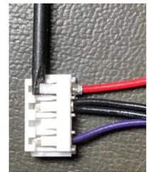
Ditch lamps flash when the horn is activated (command mode only). These four outputs are capable of driving LEDs or bulbs of low voltage. One common output may be used for either ditch lights or markers. The outputs will drive 1.5 volt LEDs or small bulbs provided by the manufacturer. Note that many LEDs and bulbs require a higher voltage if you are retrofitting the engine.
