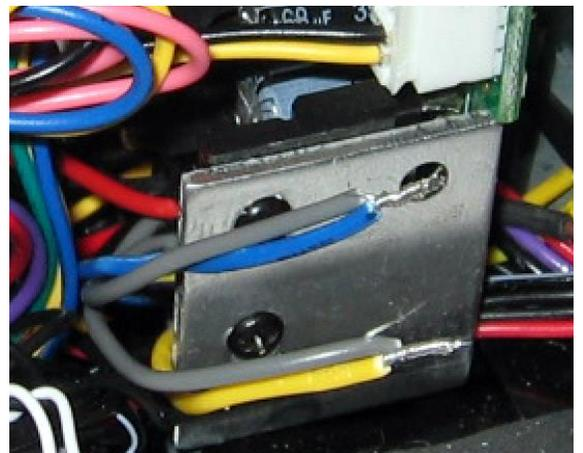
When using the temporary splices, place a piece of heat shrink (do not shrink), to protect the wires from shorting to the frame or to each other. Shown above is the temporary wiring prior to testing the engine.
