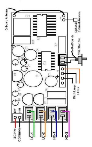
Basic directional lamps are supported by connection to LC-1 and LC-2. This configuration does not provide for Smoke, Strobe, or Cab / Marker Lamp features. When a rear lamp is not required, LC-2 may be used for those optional features.
