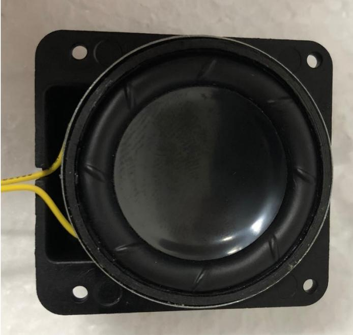
Step 2 Place the top plate over the bottom cover. There is a groove on one side. The groove face the speaker hold the speaker in place.
