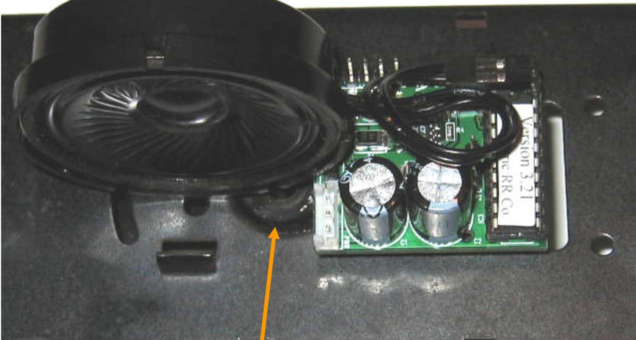
*Note: the “E” clip used to mount the truck is accessible if the truck needs to be removed.*
