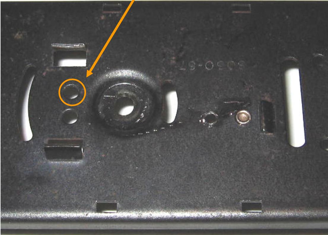
GP-9 Chassis with rear truck and “E” unit removed
