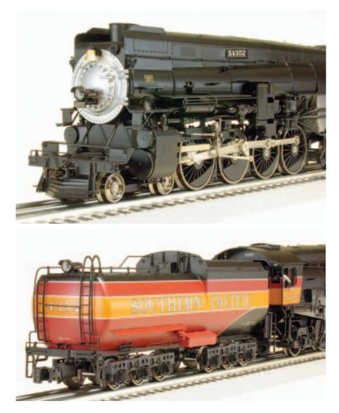
rails, air lines, and steam or water pipes are various sizes of brass wire with some of the wire spiral scored to simulate insulation wrapped around the pipes. On top of the tender's water tank are simulated wooden planks that are actually etched into a single
