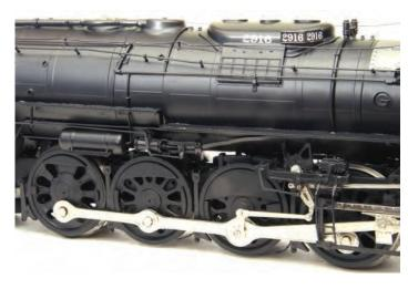
that 3rd Rail has used for years. Steel rims pressed onto the drivers give them the necessary durability needed for rolling on rails.
