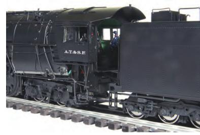
pick up the radio frequency TMCC signals directly from the track. Two sets of wipers on each tr uck are wired to the antenna lead for the TMCC receiver board. The normal design for metal steamers with TMCC uses one or more insulated wire handrails for the signal r eception antenna.
