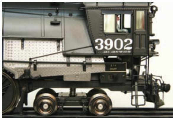
Slide switch under the cab selects steam exhaust chuff rate. Pilot details include the coupler cut lever and link to the scale dummy coupler.
